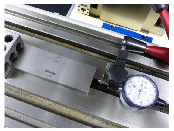
5. Move your table so that the dial indicator now plunges against the gage block and the dial indicator zeroes out:
