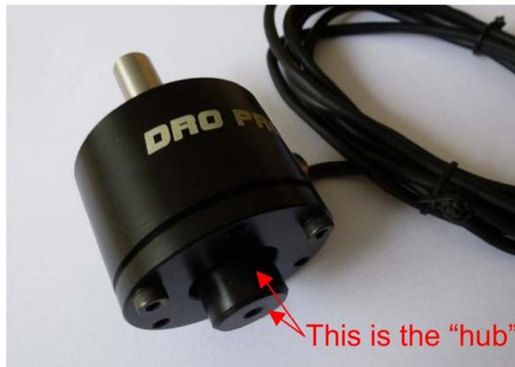
If you can't get a good enough grip on the hub, it is possible to disassemble the touch probe by removing the three 2.5mm cap screws. Work slowly and be careful to not lose the spring, which is located inside the probe. It has a tendency to 'jump out' if the probe is inverted during disassembly!
