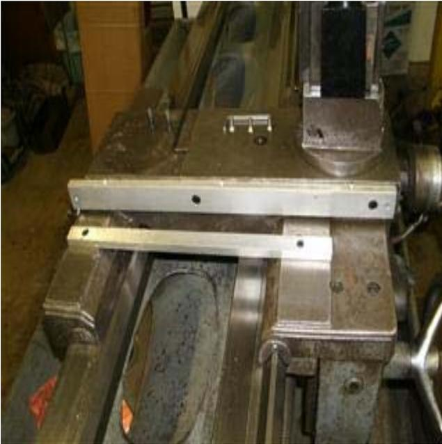
The mounting bar must be adjusted for perfect alignment in two planes BEFORE the scale is installed. Mine required only slight vertical adjustment of the scale when it was installed. Note the reader head is disconnected and the BPP is installed during scale alignment.
