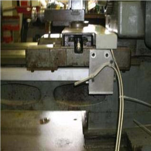
Carriage travel of this lathe is more than the 1200 mm scale can handle so a stop was fabricated. It is merely a piece of steel tubing of the correct diameter and length slipped over the clutch operating bar. Still allows full distance between centers and is not really necessary as long as the tailstock is on the ways. SOME form of hard, non removable stop is required to prevent destroying the scale from over travel! (No picture)
