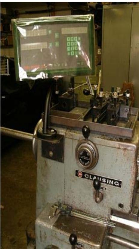
The cables from the scales are clamped securely but are still prone to getting tangled up with swarf in the chip pan as the carriage is moved. A screen door spring will be attached to keep the cables where I want them rather than piled up in the chip pan.
