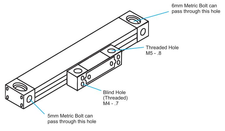
Depending on your particular kit (ie lathe vs mill, 2 vs 3 axis etc), your DRO kit will contain a mixture of metric hardware. These are the most common size components in our kits:
