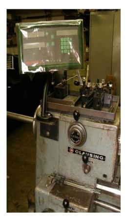
The cables from the scales are clamped securely but are still prone to getting tangled up with swarf in the chip pan as the carriage is moved. A screen door spring will be attached to keep the cables where I want them rather than piled up in the chip pan.
